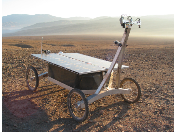
Figure 3.3: Zoë, the “robotic astrobiologist” used in the Life in the Atacama project.
